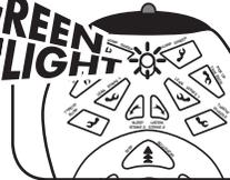
To access the Green Commands, first press the **SELECT** button once. The **GREEN** indicator light will **LIGHT AND HOLD** to confirm the selection.
