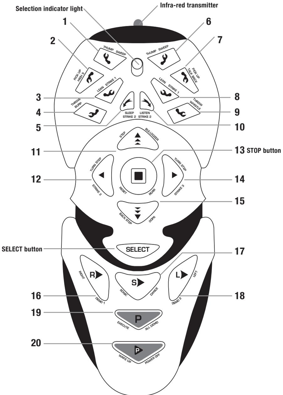
**NOTE:** The LEFT side of the Controller operates Robosapien X™'s RIGHT side; the RIGHT side of the Controller operates Robosapien X™'s LEFT side.
