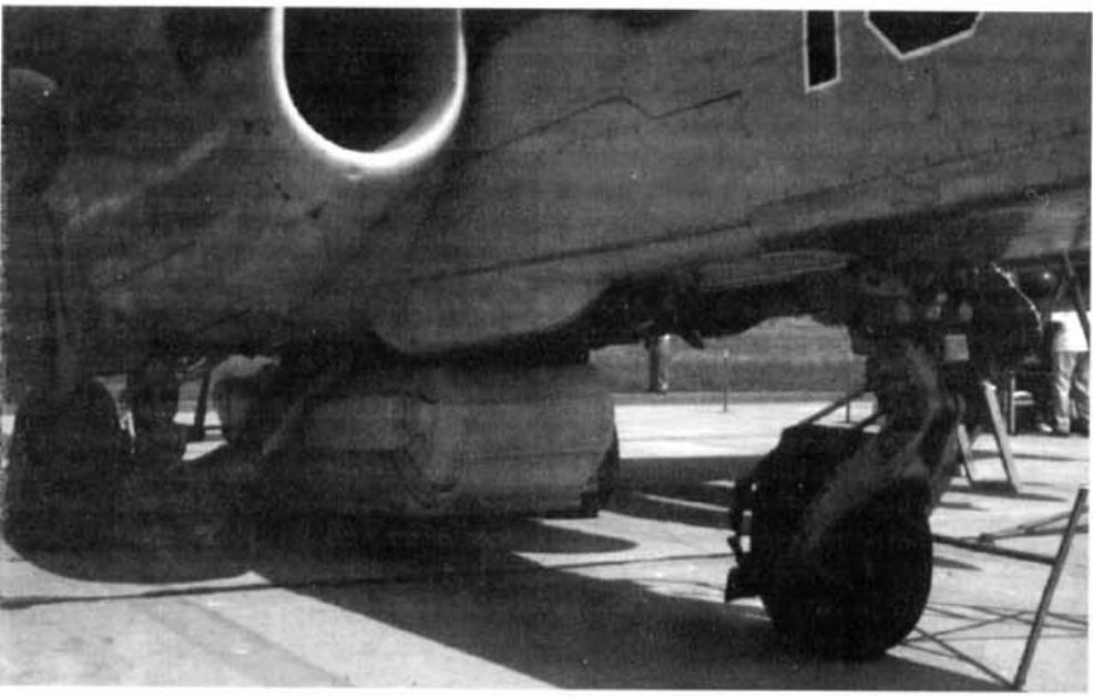
Below: GSh-2-30 (AO-17A) twin-barrel cannon under the starboard side of flat bottom of Su-25TM's fuselage. The steel screen in front of the barrel muzzles protects the fuselage skin. The big pod suspended under the fuselage contains 'Khod' FLIR.
