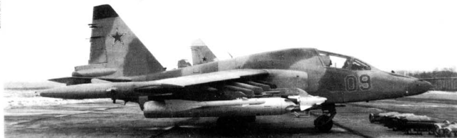
Above and below: An Su-25TM during the show for the CIS leaders in Machulishche in February 1992. 'Vikhr', Kh-29, S-25L and R-60 missiles as well as B-13 rocket launchers are carried under the aircraft wings. The unguided weapons including S-24 rockets as well as FAB-500 and FAB-250 free falling bombs are exposed in the front.
