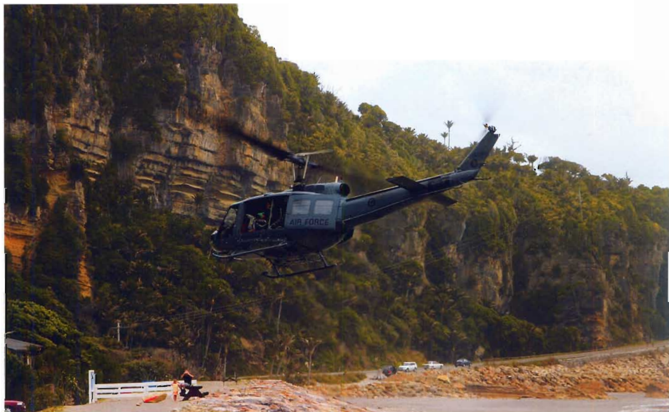
▲ A Royal New Zealand Air Force UH-1H during a search and rescue mission. A hoist and a rescue basket for picking up castaways and injured is visible behind the aircraft commander. / James Eden
