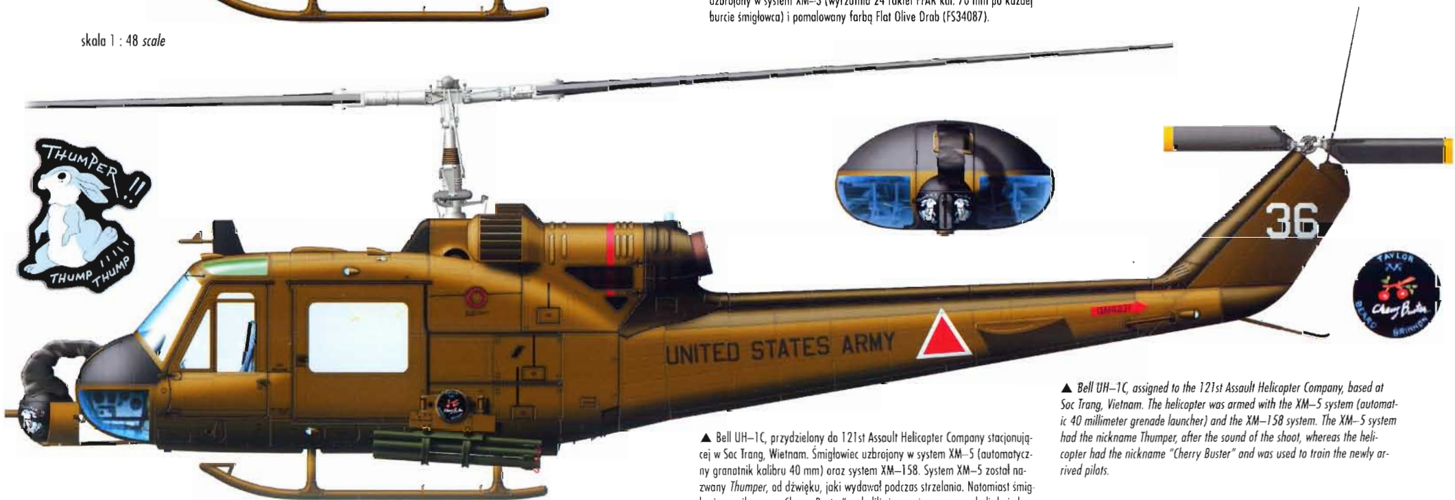
▲ Bell UH-1C (65-9533) operated by the 176th Assault Helicopter Company — Muskets, based at Chu Lai, Vietnam in 1971. The helicopter was armed with the XM-3 system (24-tube 70 mm FFAR rocket launcher on each side of the helicopter) and painted Flat Olive Drab (FS34087).
