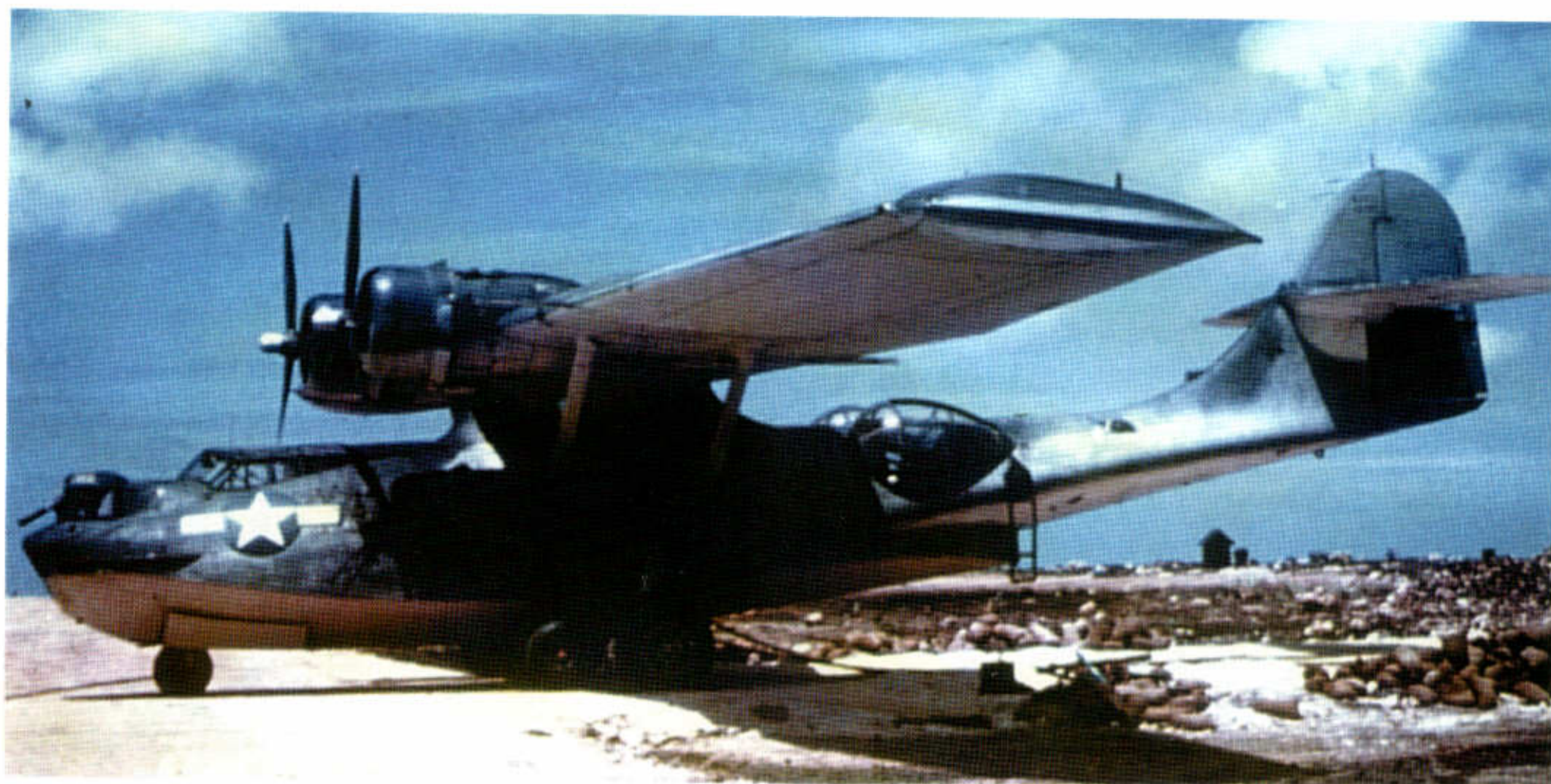
▼ Interesting painting scheme on a PBY-5A. Black was applied over the standard scheme of Blue Gray/Light Gray on upper surfaces, which resulted in a three-tone scheme. The camouflage was used at the end of the war in the Pacific / National Archives
