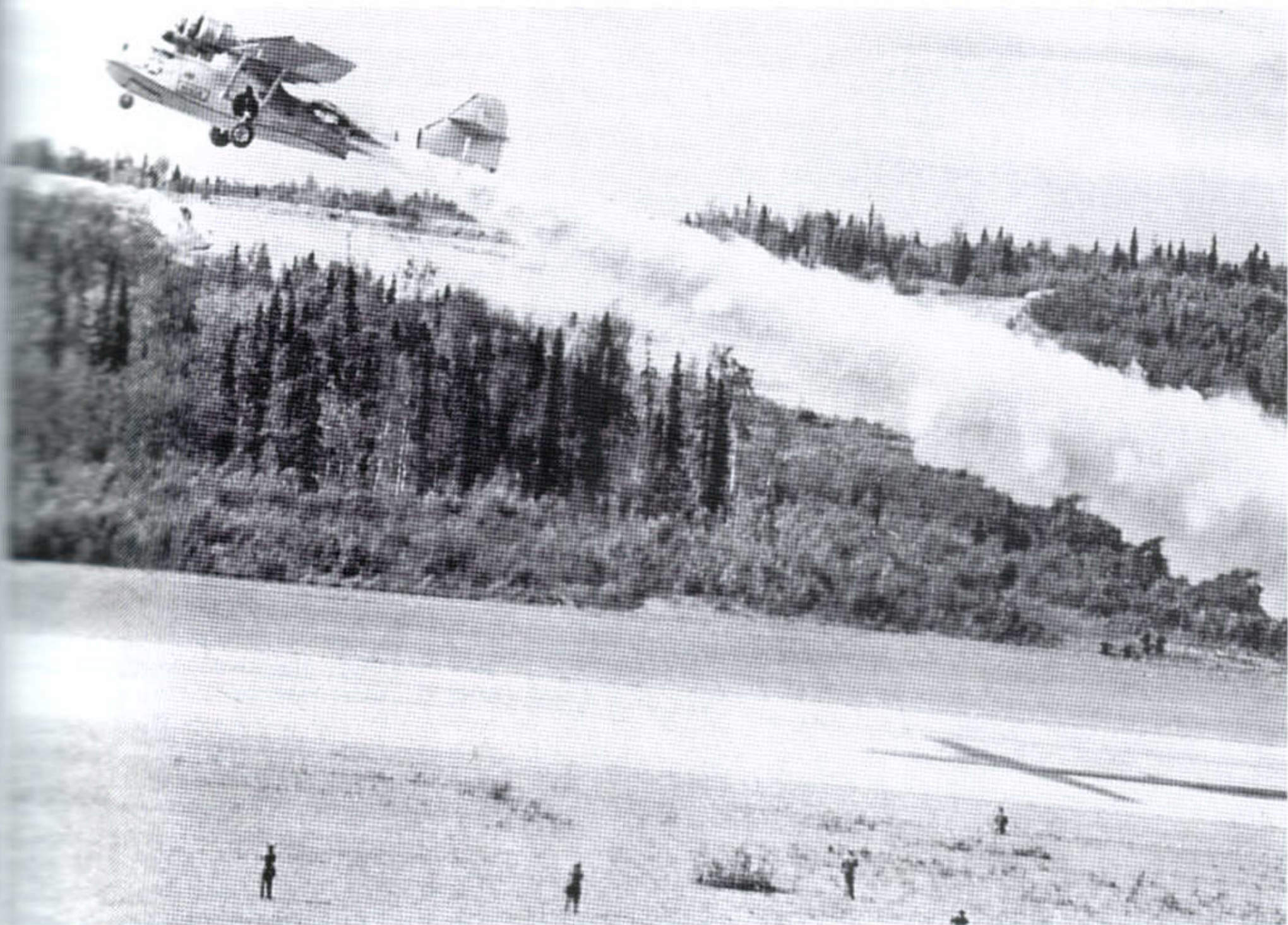
▼ OA-10 of the 10th ERS shows JATO. Usually two such boosters were attached under wings, in order to shorten and facilitate the take-off / National Archives
