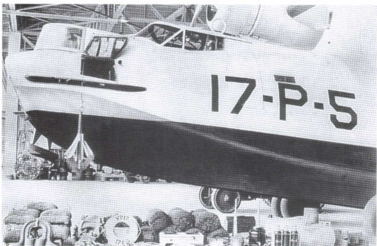
▼ The anchor was stored in a special compartment in the port side of the hull. An instruction was affixed on the hatch / National Archives
