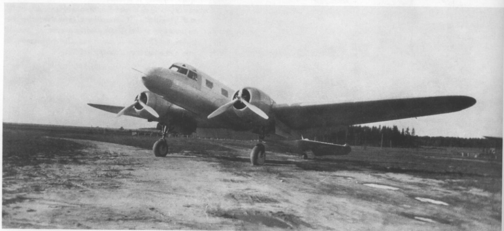
▼ Airline derivative of the SB, ANT-35 for 10 passengers / via V. Kulikov
