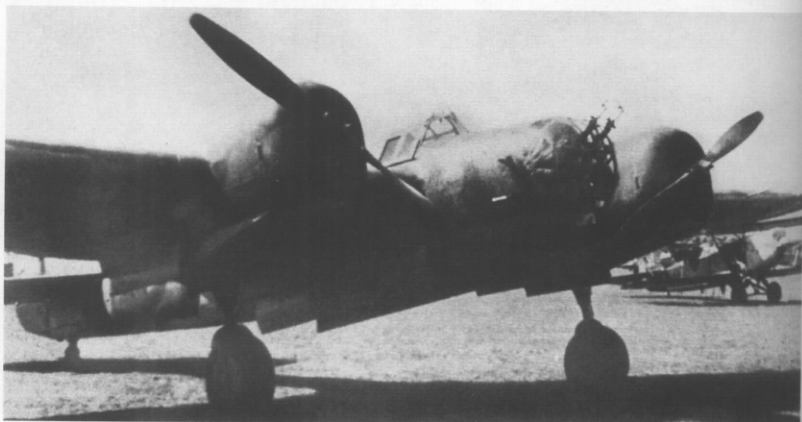
► Another camouflaged Spanish SB-2M-100A. Note the ShKAS machine guns in the nose / via V. Kulikov
