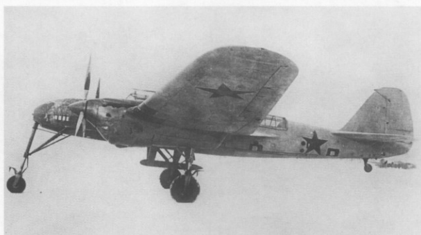
◀▼ „Pterodaktil” — SB with experimental tricycle undercarriage. Note the special frame to which the main wheel legs were attached. These could be re-positioned backwards-forwards in order to find optimum position relative to the aircraft centre of gravity / via V. Kulikov
