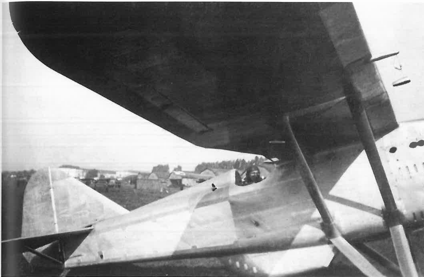
Kabina i dysza pomiarowa na skrzydle. Cockpit and the testing tube on the wing.
