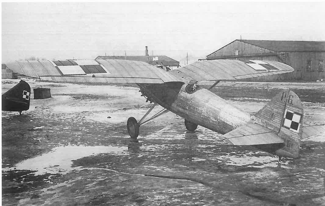
Below: The P.6 at the factory with weights stenciled on the rudder: WP1340, WW865, CP268, CU207. Note the tail of the P.7 prototype.
