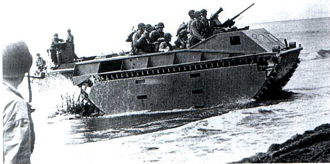
Uzbrojona (dwa karabiny maszynowe) amfibia LVT-1 z 1. lub 2. Batalionu Amfibii używana w walkach na Guadalcanal. LVT-1 of the 1st or 2nd Amphibious Tractor Battalion was used in initial assault and was armed with two machine guns. [U.S. Army]
